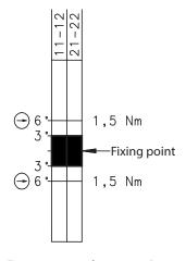
Fixing point in the range  $0^{\circ}$  ...  $270^{\circ}$  freely selectable
